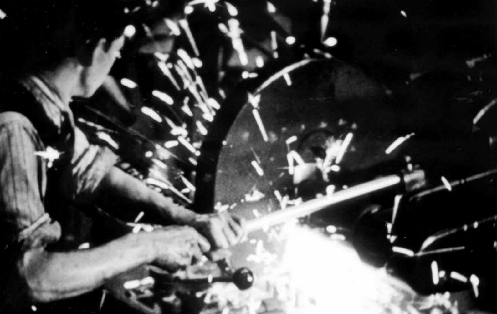
Jimmy Carman cutting through a "sausage type" length of compression springs which would then become individual springs with ends virtually ground square.
